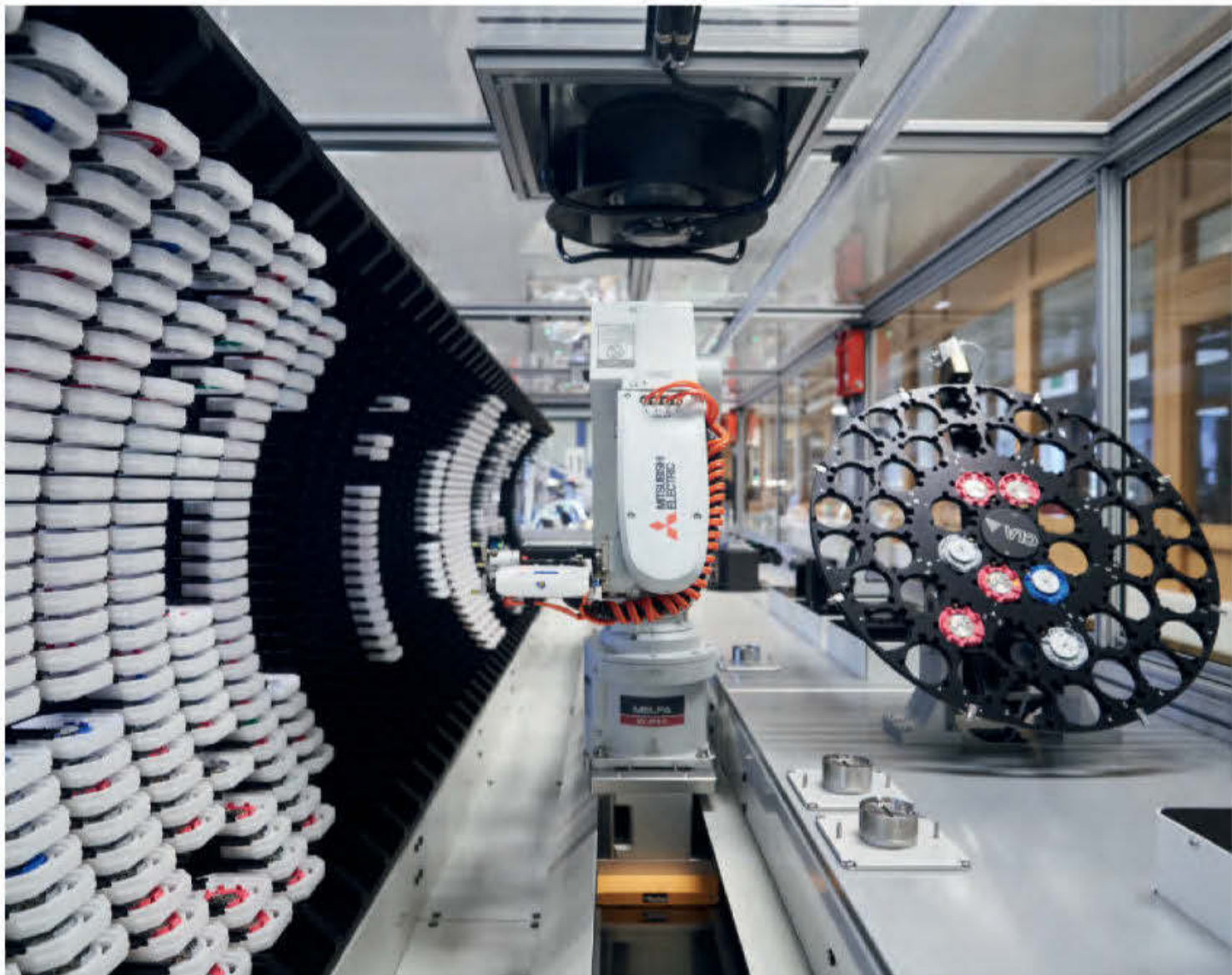
Above: Assembled watches are quality-checked by the CLAchronométrie. Its robot arm scoops up each cartridge and tests its contents on amplitude, winding, and pusher operation.
