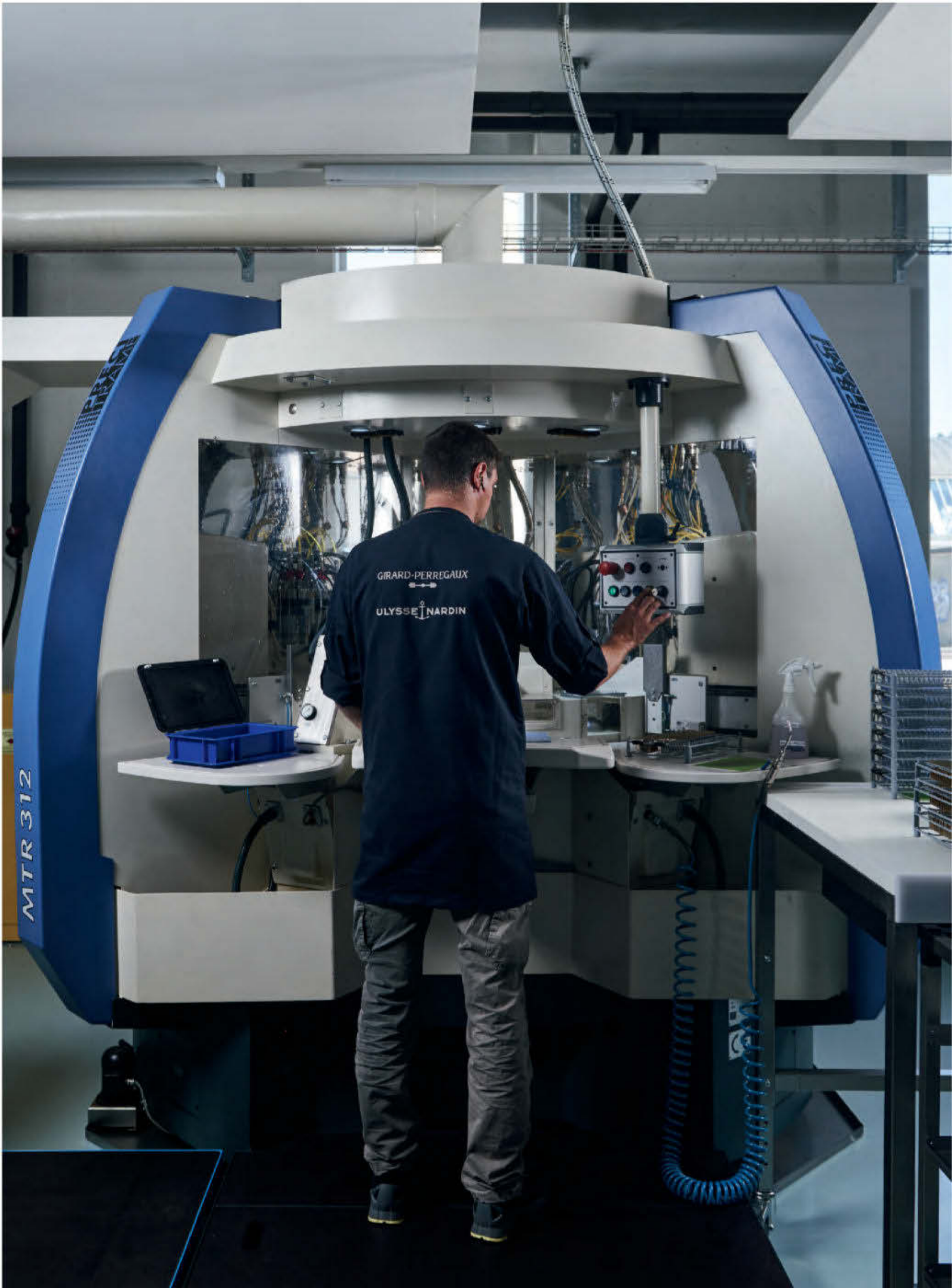
This 12-position machine makes adjustments to mainplates that form the base of each movement.
