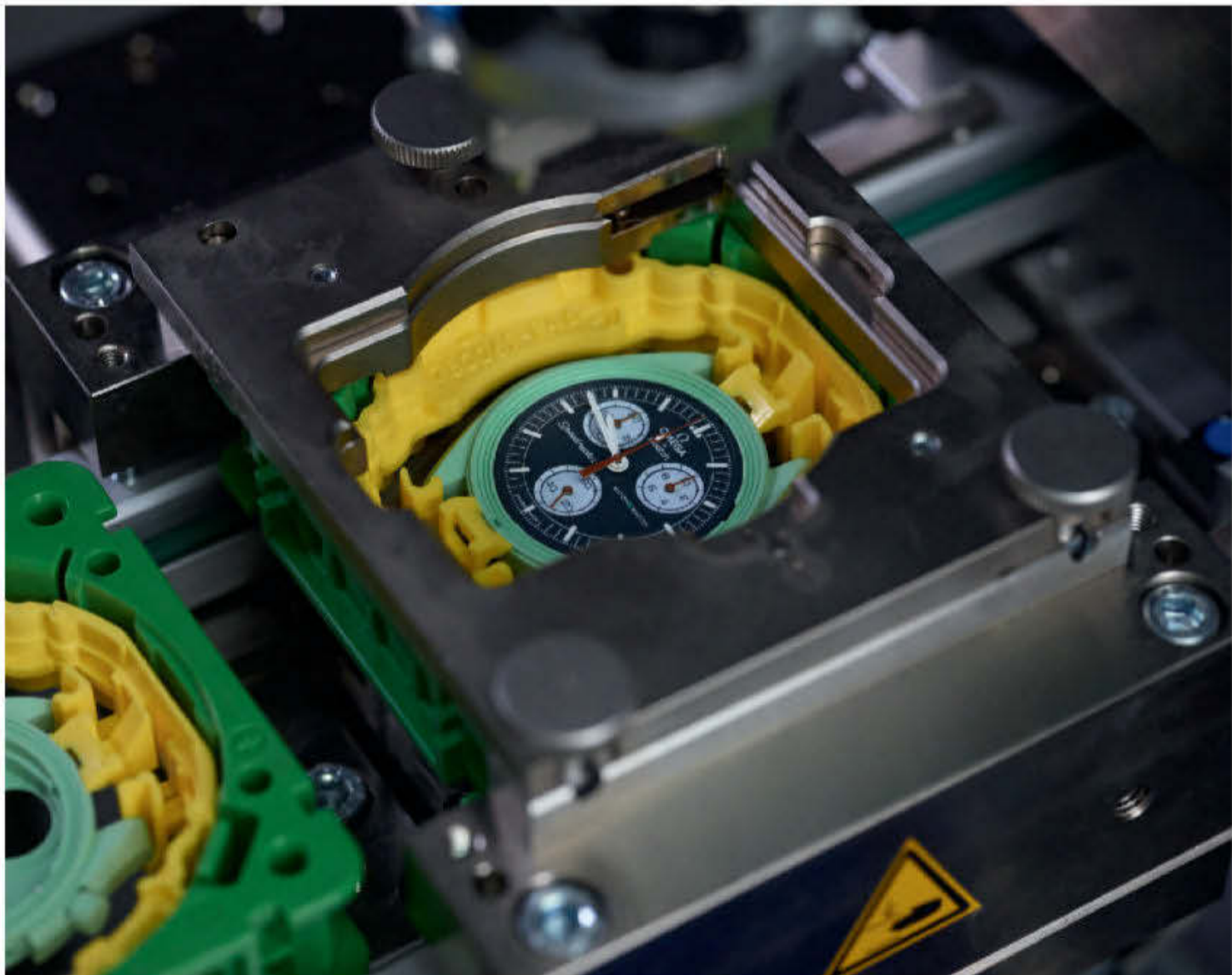
Above: An automated assembly line drops the completed movements for a Mission to Earth MoonSwatch into a Bioceramic case, ready for a robot arm to place the biosourced glass.
