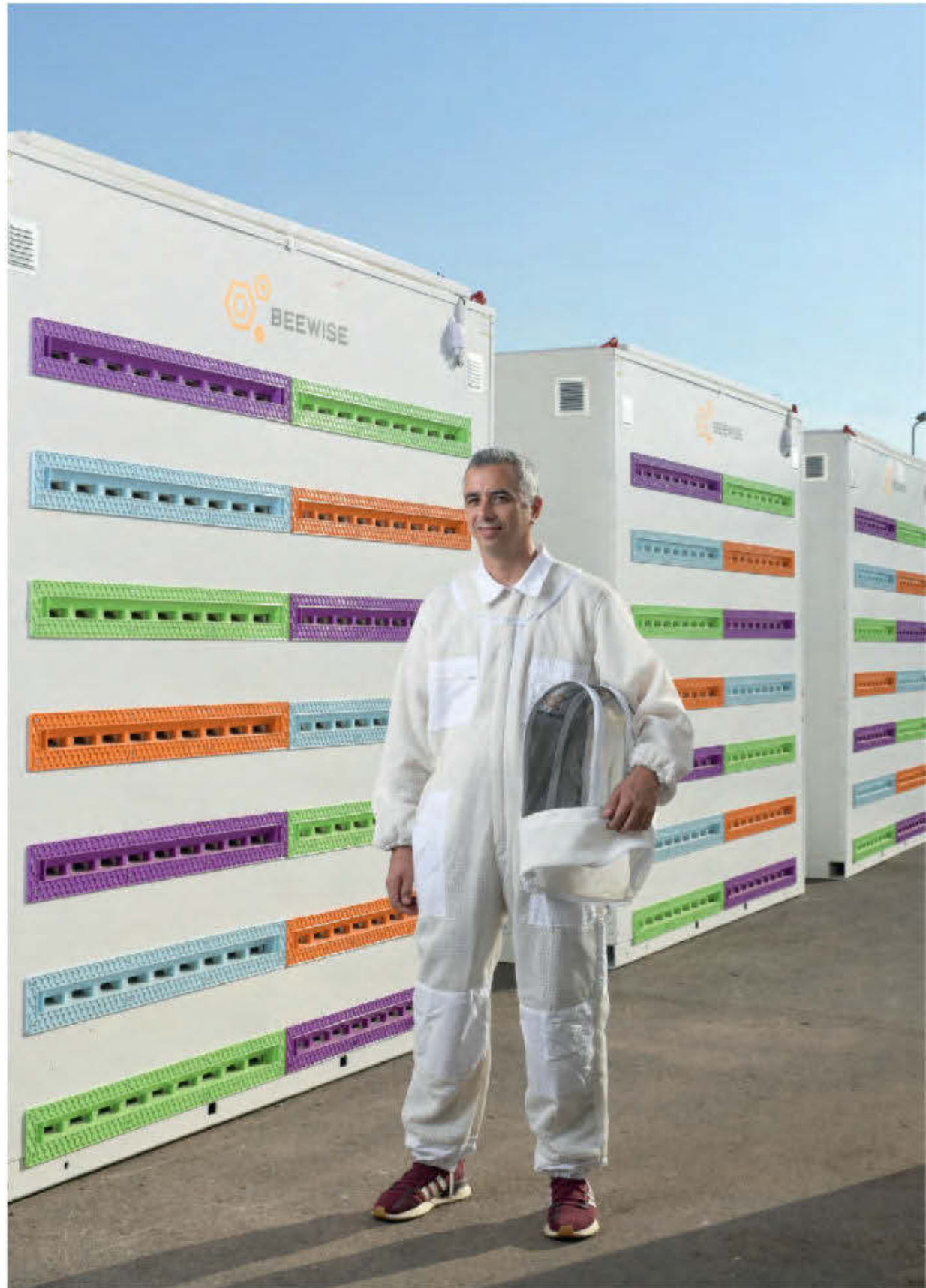
Saar Safra, CEO and cofounder of Beewise, in front of his robotic hives, which can monitor a colony's health, adjust the temperature, and detect pesticides.
