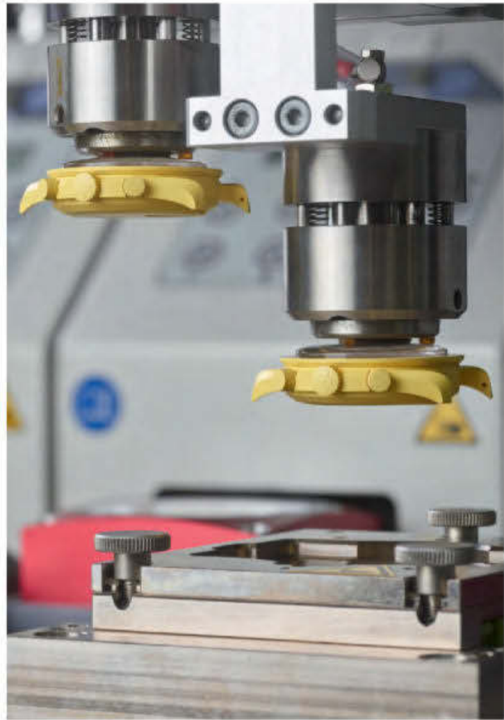
Above left: The original Omega Moonwatch, next to a new MoonSwatch Mission to the Sun. Above right: Robot arms lift completed timepieces to the next stage: strap fitting.
