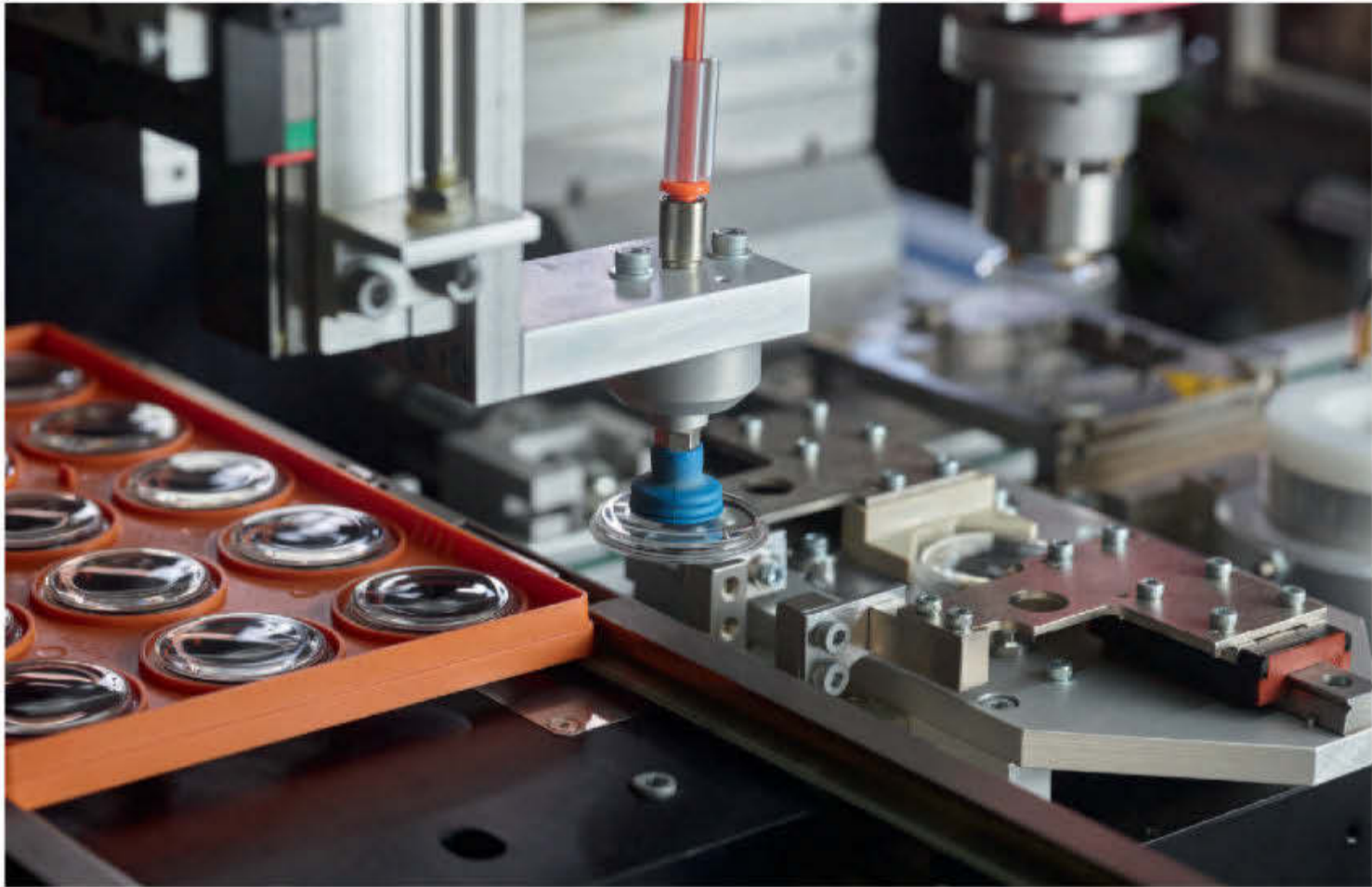
Above: A tray of biosourced glass ready for installation on MoonSwatches. Even this delicate operation is performed by robots on the fully automated production line.
