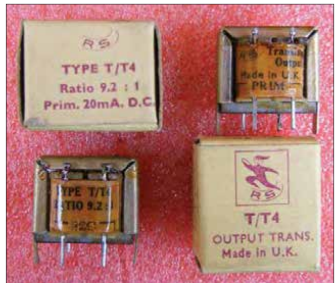
Fig.61. Transformer for the little class-A amp in Fig.60. I've had one of these in my junk box, sorry: 'strategic research and development inventory', since 1972.
