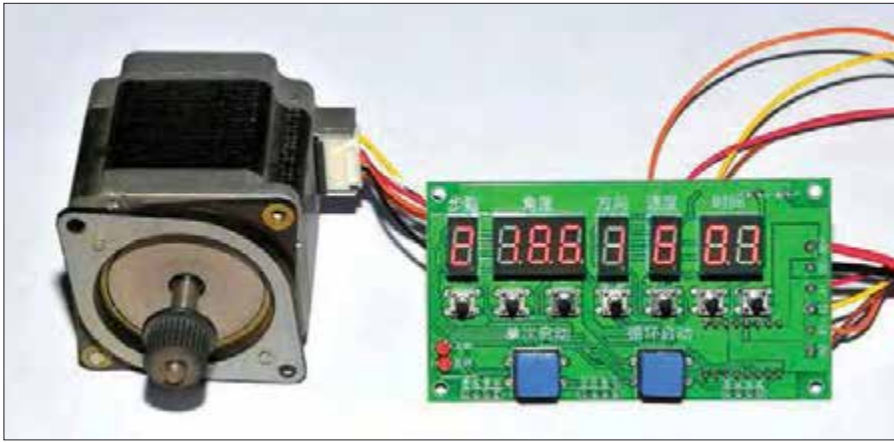
Fig.7 This standalone programmable controller is a very easy way of getting a stepper motor up and running. Speed, direction and rotational angle can all be set, and the module has the ability to store nine programs that can be run automatically in sequence.
