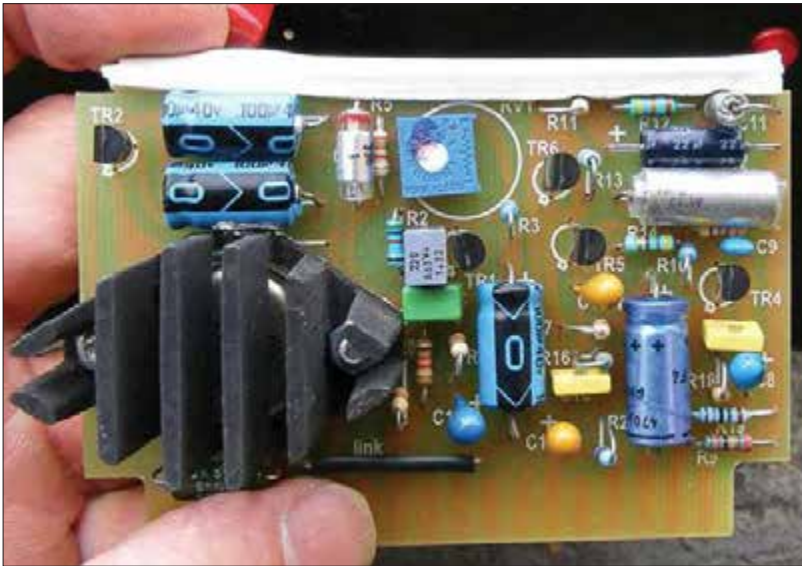
Fig.54. Neve BA238 output driver board. Note the uses of a TO3 output transistor: bomb-proof, good-sounding over-engineering.
