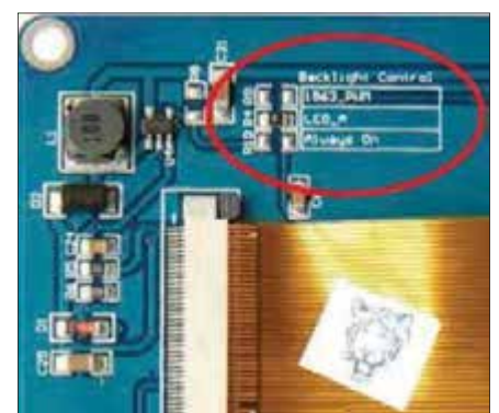
Fig.3. On some SSD1963 tft modules, you may need to modify the backlight control. If applicable, remove the ‘LED-A’ short, and ensure the ‘1963-PWM’ link is shorted instead.
