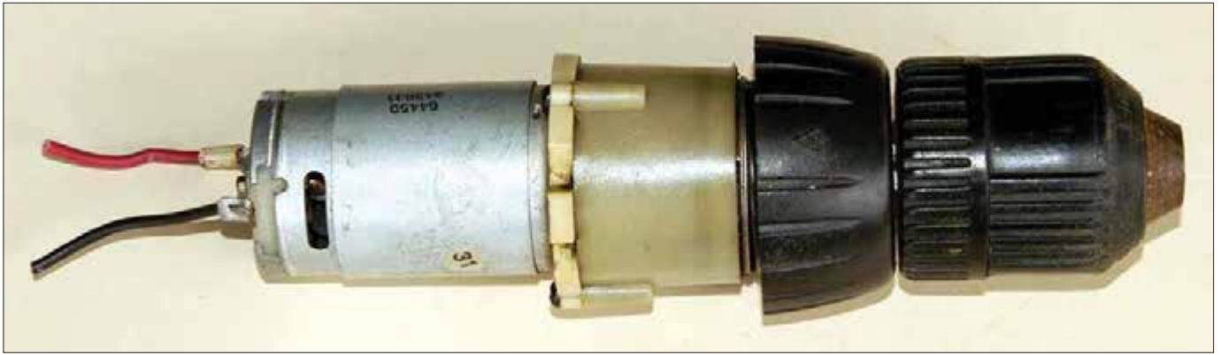
Fig.3. The motor/gearbox assembly from an old battery-powered electric drill. These can be obtained at low/no cost and have excellent torque. The mechanical connection to the output can be made by clamping a shaft in the chuck.
