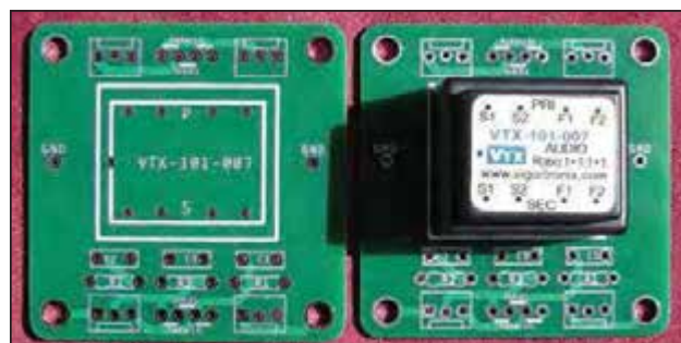
Fig.39. The Vigortronix/OEP transformer mounting boards. These allow series/parallel linking, Zobel networks and the use of Molex connectors.
