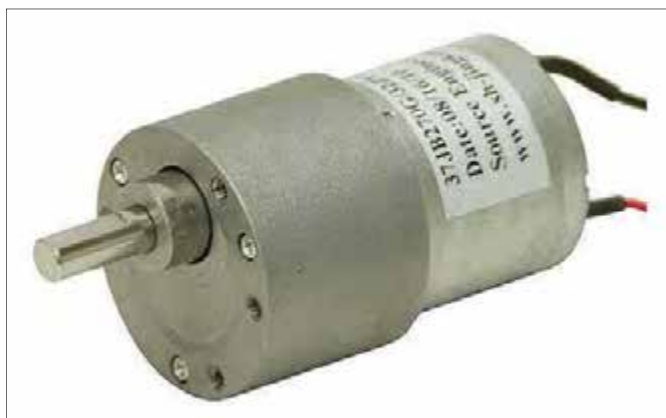
Fig.1. A gearmotor – note how the gearbox is attached directly to the end of the motor, giving a compact assembly. The typical D-shaped output shaft can be seen. This gearmotor is a 24V design that rotates at a no-load 25 RPM (150°/s). Cost is just £6.
