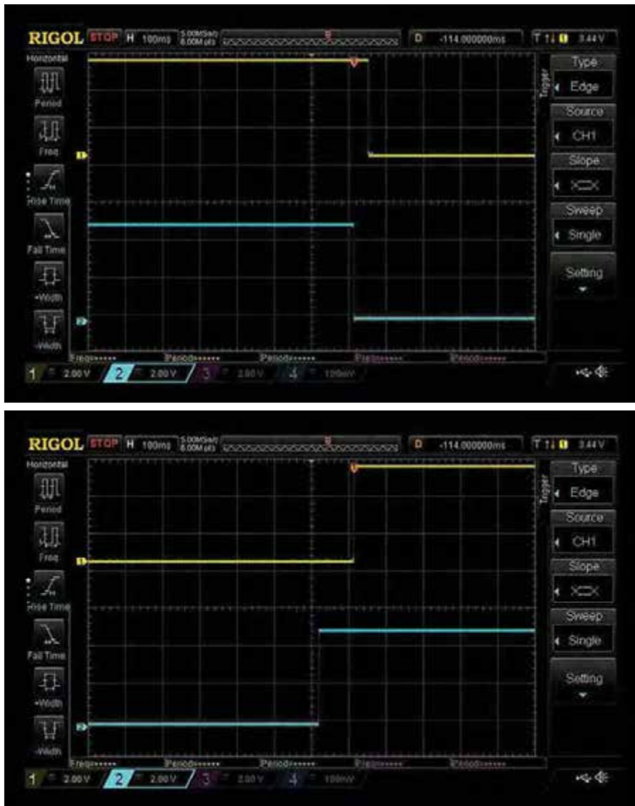
Fig.8. 30-click device: a) (top) turning the knob one click anticlockwise; and then b) again.
