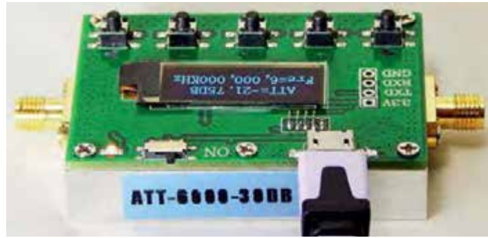
The 6GHz digital attenuator from Banggood has an OLED screen and weighs about 57g.
