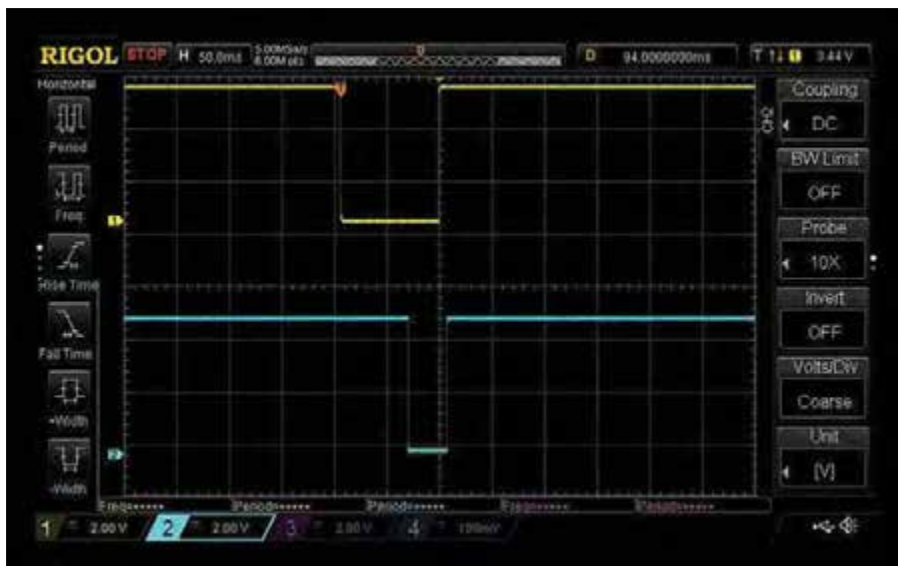
Fig.9. 20-click device: a) (top) turning the knob one click clockwise; and then b) (bottom) turning one click anticlockwise.
