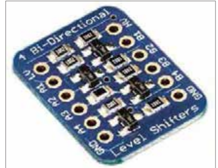
Fig.5. Pre-built level shifters are available, but it is also possible to build your own very easily – see Fig.6.
