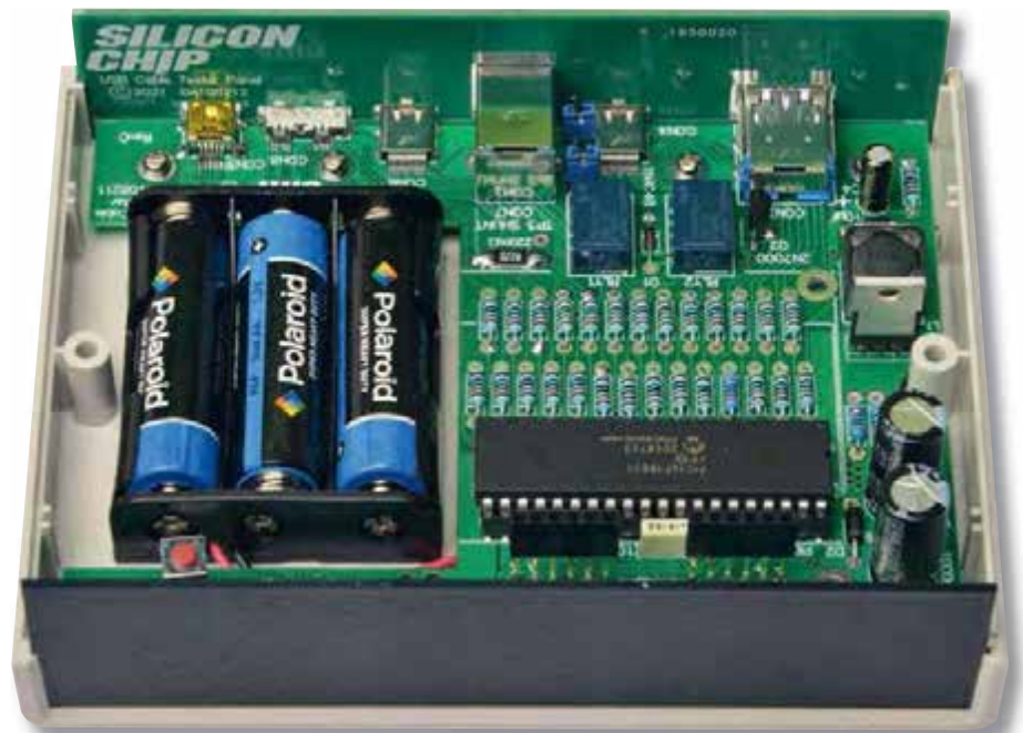
The completed USB Cable Tester photographed from the front and rear. This shows that all connections are made from the front of the case. One tactile switch is raised so it can be more easily accessed through a hole in the lid.
