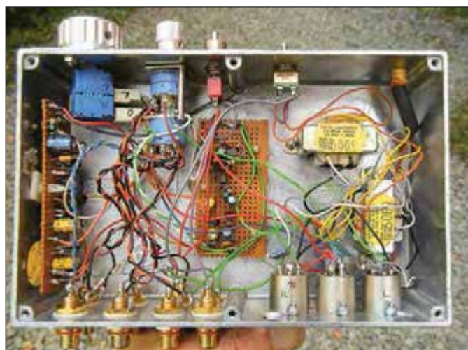
Fig.37. Studio monitor control unit with Sowter 5069 Mumetal/M6 output transformers. The Zobel network is 22nF and 1.5k \Omega . This is the same transformer that we discussed in Fig.30 in Part 2 .
