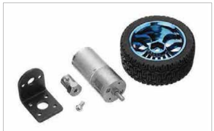
Fig.2. A gearmotor, mounting bracket, coupling and wheel. Gearmotors are ideal for driving wheels on moving robots and similar – this gearmotor operates on 6V, draws a loaded 0.5A and rotates at 100 RPM. Cost is £11. (Courtesy Banggood)
