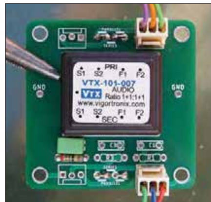
Fig.42. Line-output board with parallel-connected VTX-101-007 transformer. The Zobel network is 1.3kΩ and 6.8nF.
