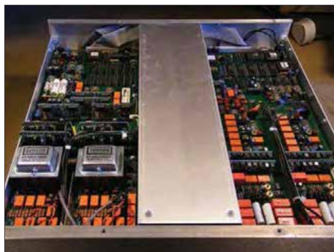
Fig.38. Custom-wound Jensen output transformers (lower left) in the Audio Precision SYS-2712 analyser. This transformer balanced output has the lowest distortion I've ever seen. It has to, since it is the system by which other amplifiers are measured.
