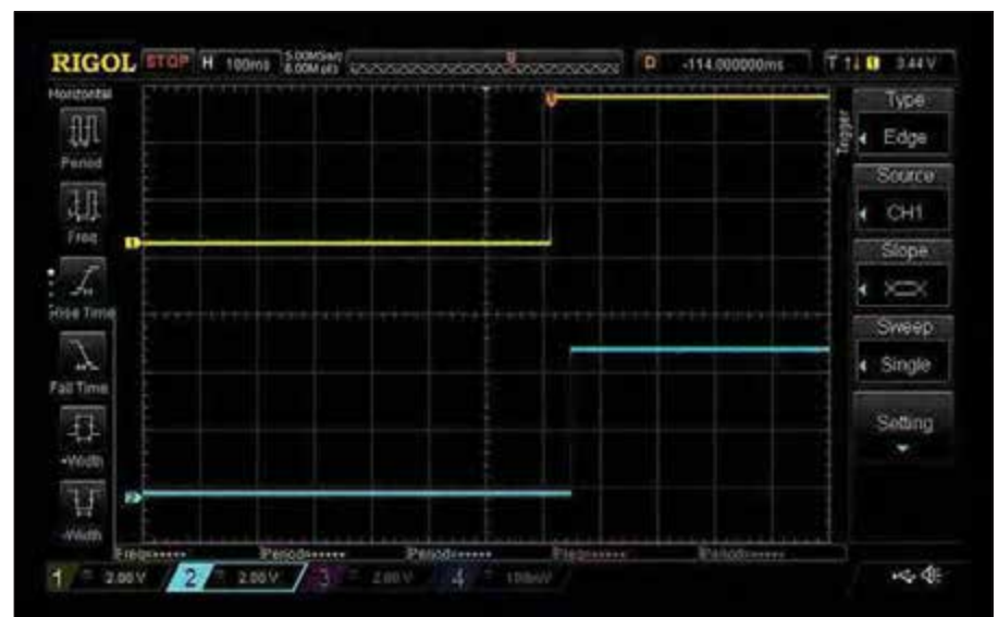
Fig.7. 30-click device: a) (top) turning the knob one click clockwise; and then b) again.
