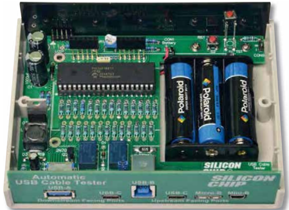
The completed USB Cable Tester photographed from the front and rear. This shows that all connections are made from the front of the case. One tactile switch is raised so it can be more easily accessed through a hole in the lid.
