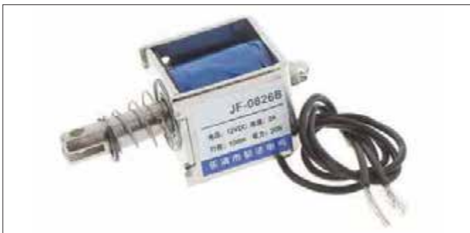
Fig.8. A typical general-purpose solenoid with a spring return. This one is for use on 12V, with a continuous current draw of 2A and a maximum pull of 20N (about 2 kg force.) Cost is low – only about £4.
