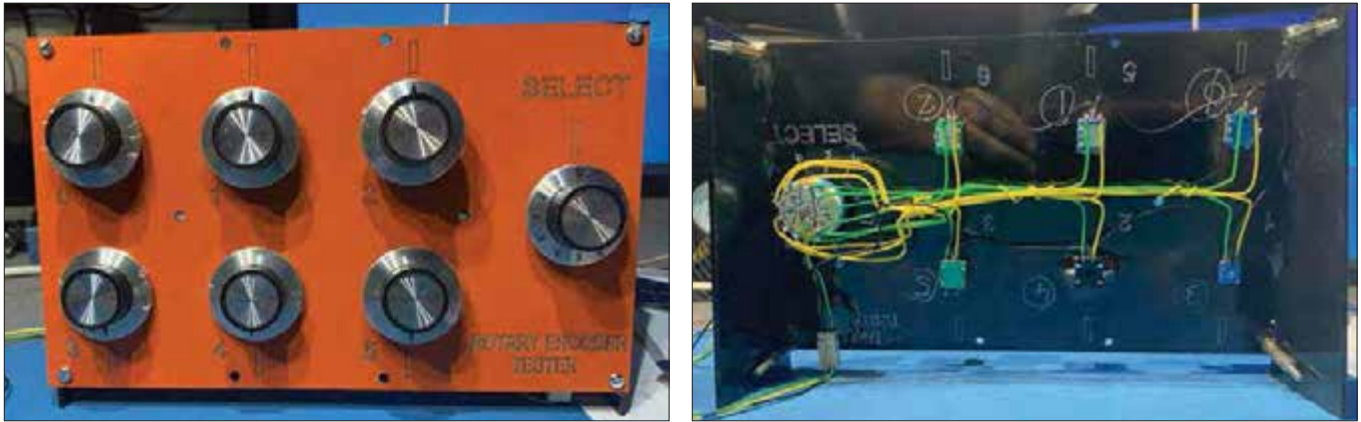
Fig.6. Testbench to evaluate six different rotary encoders. (Image: Joe Farr)
