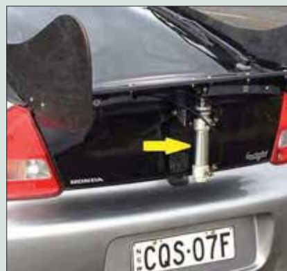
Fig.10. A trial rear aerodynamic air brake on a road car. When braking, the panel between the side fins was rapidly raised through about 80 degrees. The speed of the required erection, and the forces involved, meant that no off-the-shelf electrical actuator could do it – no matter the leverage applied. But a pneumatic cylinder (arrowed) could. And the result? At very high speed the brake was excellent – but unfortunately, at legal speeds, it was rather weak. Oh, if only to drive every day in Germany...
