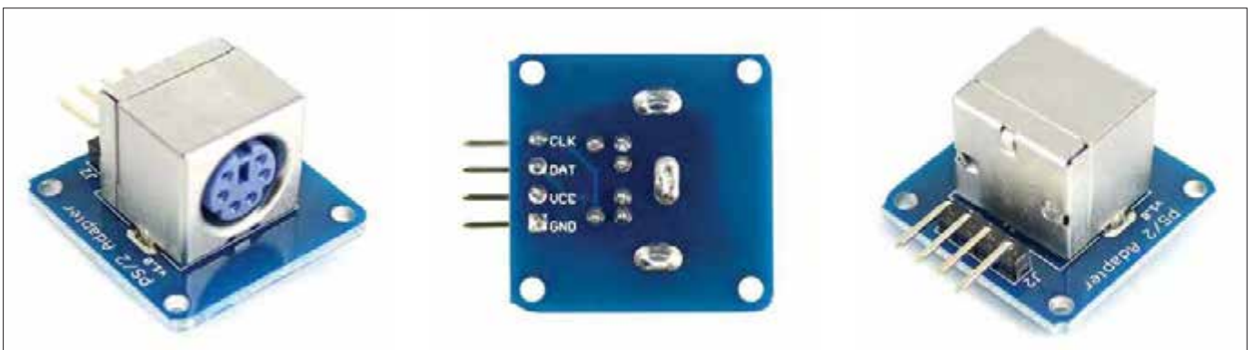
Fig.7. A PS/2 breakout board like this one makes it easy to connect the PS/2 keyboard to the level-shifter.
