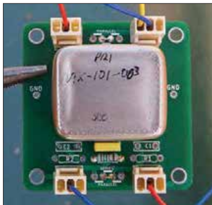
Fig.41. VTX-101-003 Microphone transformer with screening can showing series-connected windings. The Zobel values are 680pF and 15kΩ. The VTX-101-007 with secondaries in series is wired the same way with a Zobel of 13nF and 1.8kΩ.
