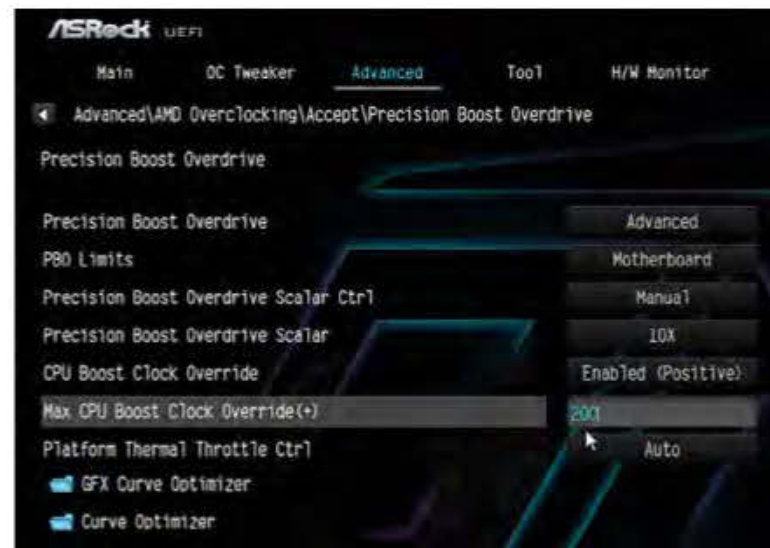
Our PBO settings enable the CPU to add another 200MHz to its frequency if there's enough power and thermal headroom
