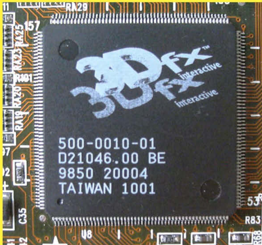
A close-up of one of the texture mapping units found on Voodoo2 cards – the 'BE' shows that it's a 'Bruce' chip. Photo credit: Stonda, licensed under CC BY SA 3.0
