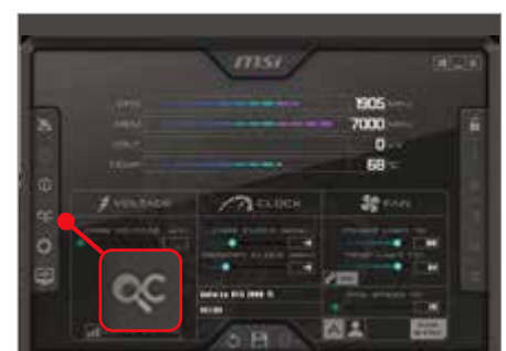
MSI Afterburner's OC Scanner lets you overclock your graphics card with one click
