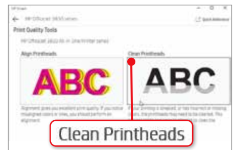
Use your printer's software to regularly clean its print heads and extend its life
